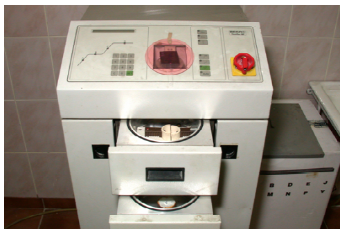
Figura 17. Aparat de topire- turnare programabil BEGO-NAUTILUS
